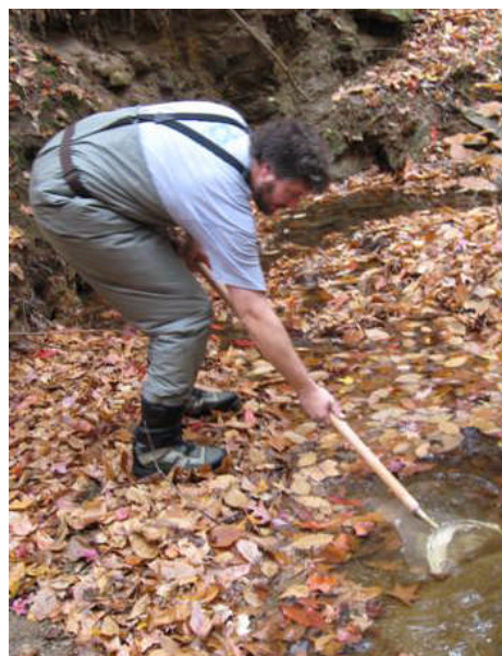
Benthic Sampling using the "jab" technique
