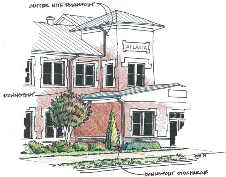
A typical small commercial roof downspout is directly connected to the site stormwater collection system
