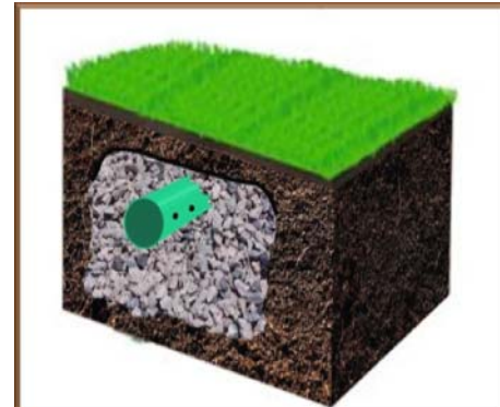
A modified French drain can be added to a small commercial site to blend into the overall site plan.
