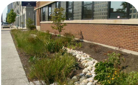
Bioretention areas can be designed to fit into tight urban spaces.
