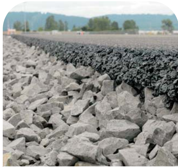
Permeable asphalt (first developed in the 1970s) consists of standard bituminous asphalt in which fines have been screened and reduced, allowing water to pass through small voids. Photo courtesy of www.socwisconsin.org .
