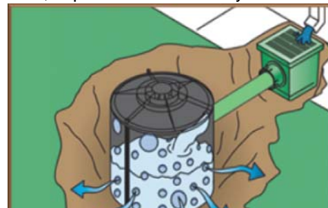
A dry well can be added to a small commercial site to help direct rooftop runoff to infiltrate in the ground.
