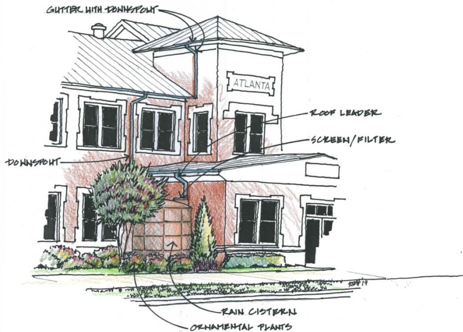
A cistern intercepts downspout runoff, and outlets to the adjacent landscape area
